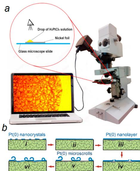
**Fig. 1** Optical microscopy and microscroll formation process. (a) Schematic and actual setup for *in situ* optical microscopy to observe tube formation on the Ni surface using a drop of  $\text{H}_2\text{PtCl}_6$  solution. (b) Different stages of Pt(0) microscroll development (i)–(vi), from Pt(0) nanocrystals and nanolayer formation to the creation of Pt(0) microscrolls on the Ni substrate.
